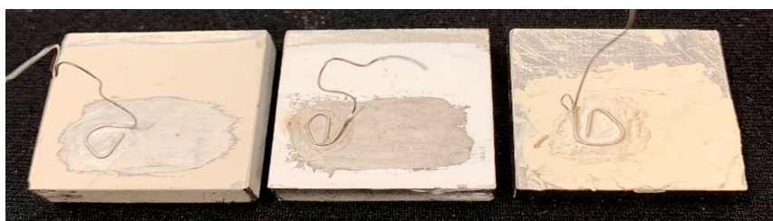
Figure 12. Bismuth titanate, lithium niobate, and organic bismuth titanate film transducers (left to right). Good adhesion was observed for extended periods of time. One film transducer is still working normally after several years of use [7].
