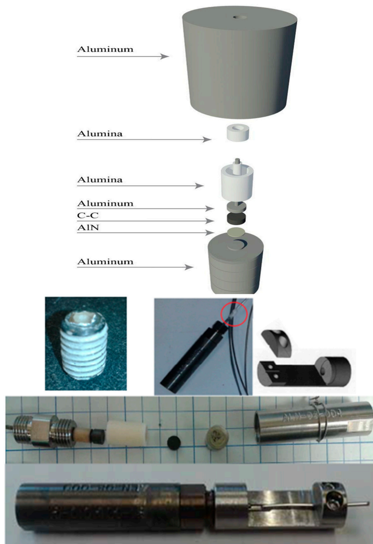
Figure 8. Photos of the fixture inserted into the Massachusetts Institute of Technology (MIT) reactor [31].
