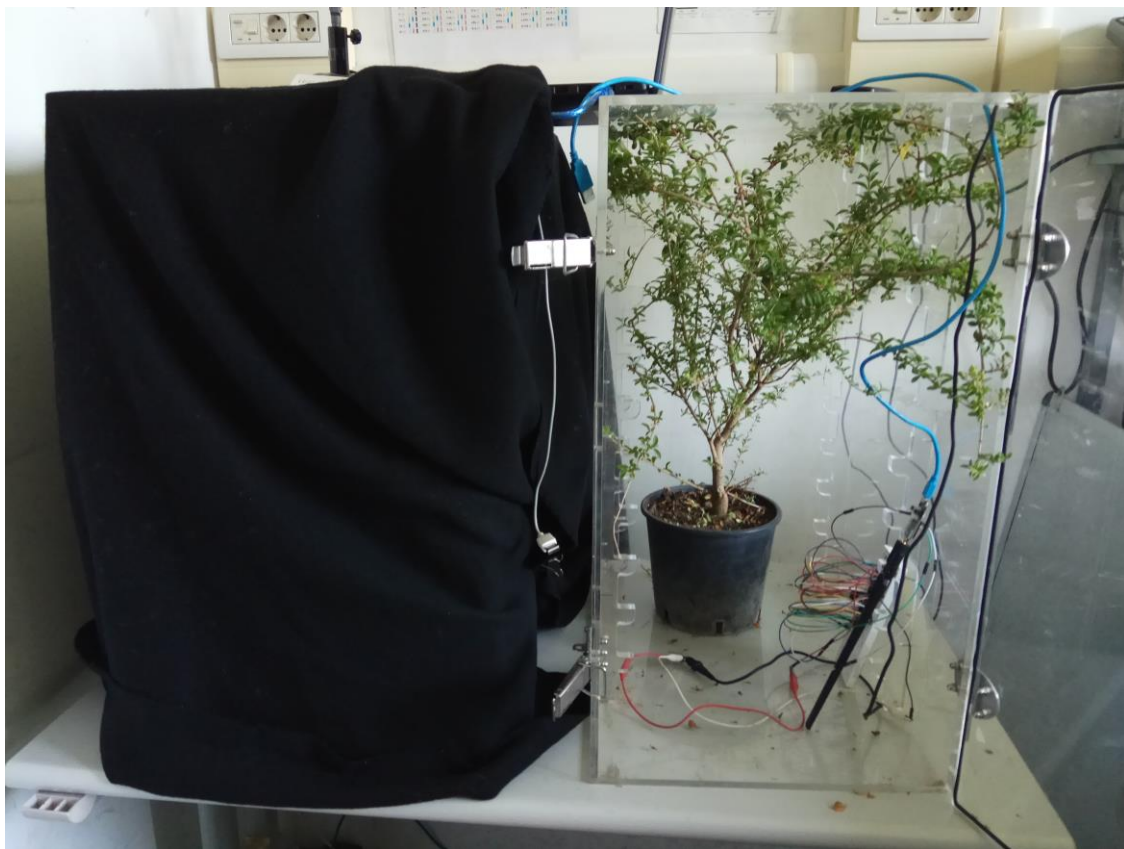
Figure 2. WSN test of plants enclosed in transparent boxes in order to simulate transport inside lorries. The transparent box shows an enclosed European privet. WSN and its antenna are also visible inside the box. The box is endowed with a series of holes for air circulation.
