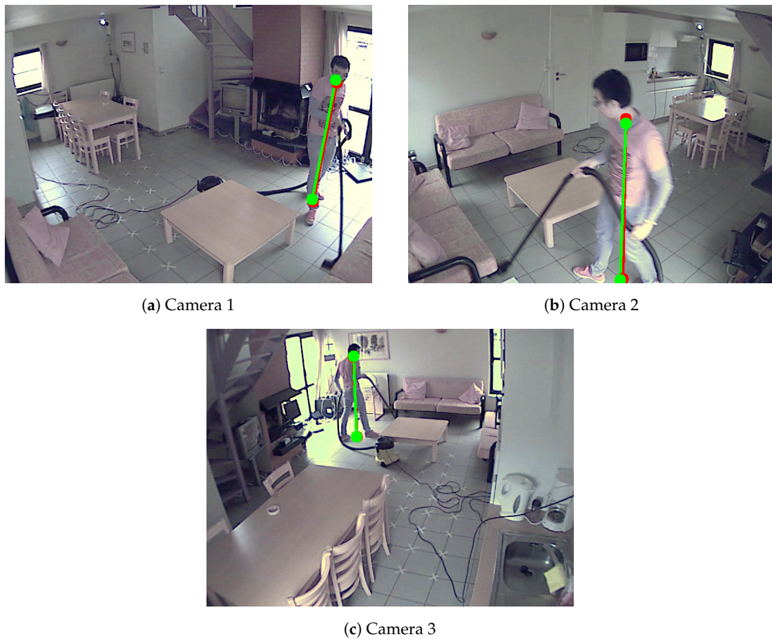
Figure 4. Example of detected the bottom and top positions of the pedestrians of Camera Network 2—single person doing household work in an kitchen room. Red color represents detected positions by the human pose estimation method. Green color represents the detected reprojected positions.
