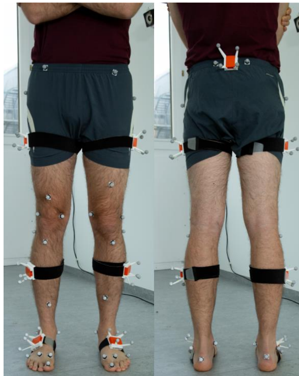
Figure 1. Schematic preparation of a subject with retroreflective markers and inertial measurement units (IMUs) inserted into rigid boxes equipped with additional markers. In the actual study, the markers on the pelvis were placed directly onto the skin. Furthermore, the subjects in the present study had to wear shoes.
