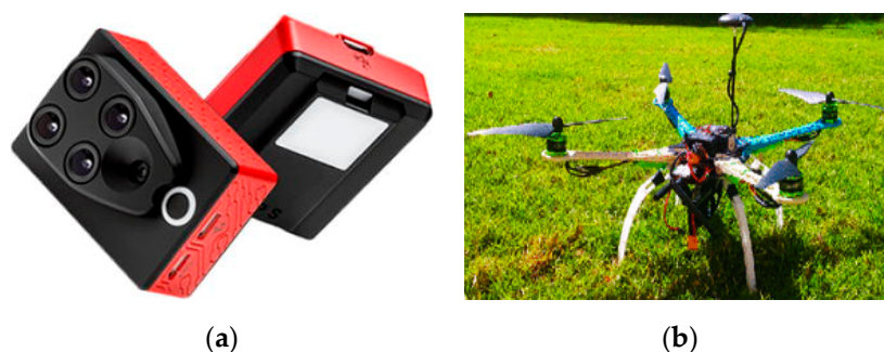
Figure 6. Examples of multispectral sensors for monitoring crop data [50]: (a) a multispectral sensor for crop discrimination and (b) an airborne multispectral sensor for assessing nitrogen nutrition [51].
