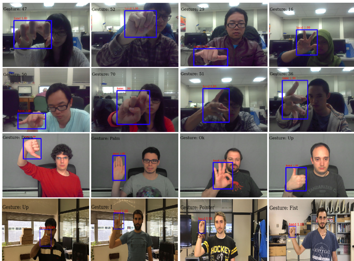
Figure 9. Some examples of hand detection and recognition results using our proposed architecture on different datasets. The first row contains images from the LaRED dataset [46]. The second and the third rows contain images from the simple and complex TinyHands datasets [47], respectively (best viewed in color).
