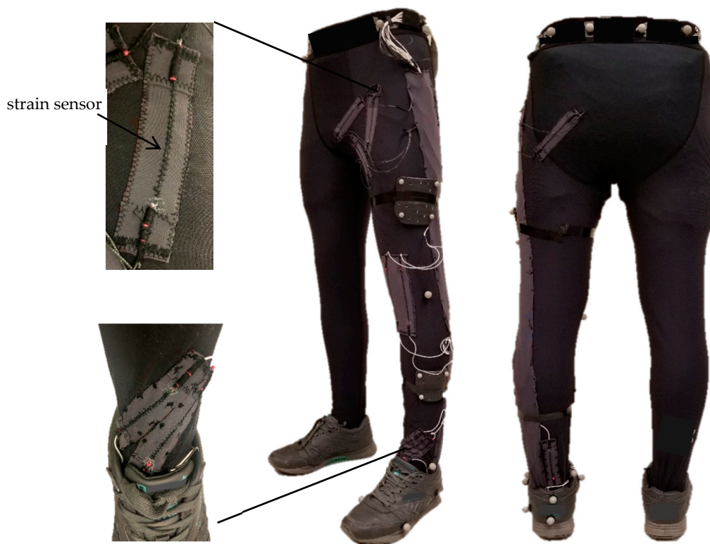
Figure 3. The fabric-based strain sensors and motion tracker markers mounted on the left leg.
