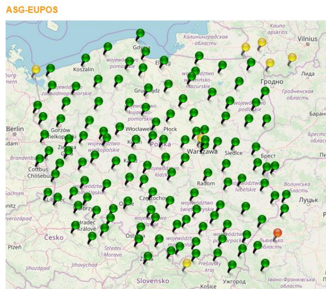
Figure 21. Distribution of the GNSS reference stations of the ASG-EUPOS network. ( www.asgeupos.pl [11]).
