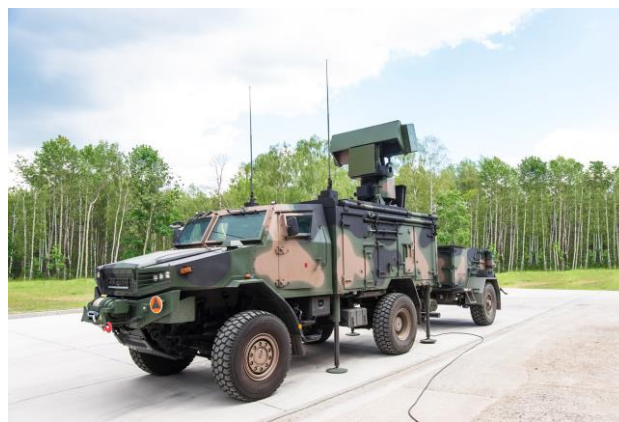
Figure 4. Redeployment-capable radiolocation station BYSTRA ( www.pitradwar.com ) [9].
