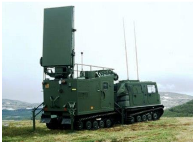
Figure 1. ARTillery HUNting Radar ( www.radartutorial.eu ) [8].
