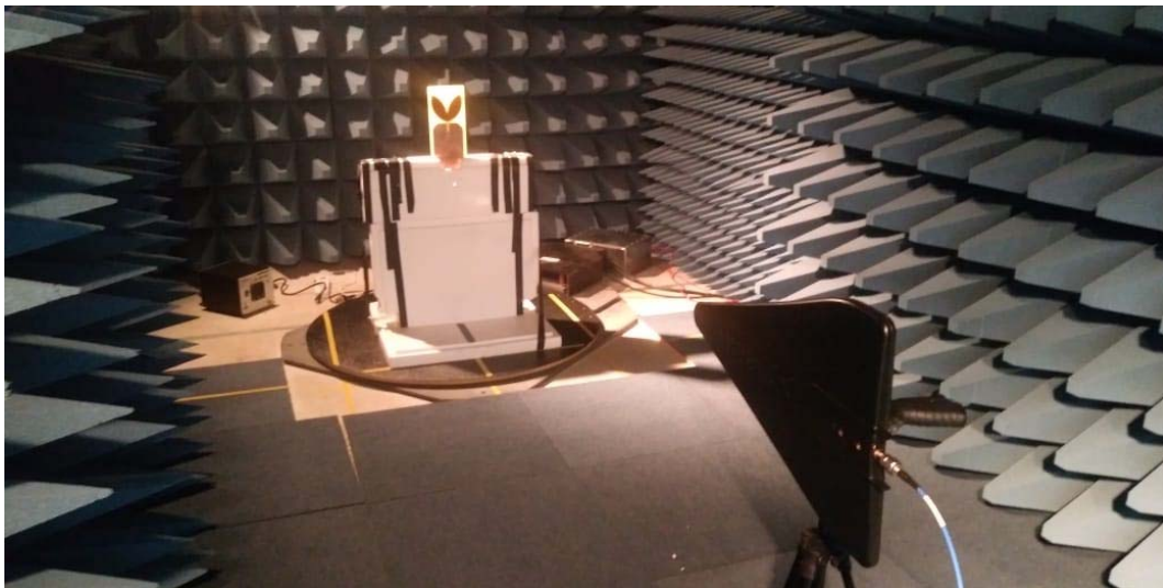
Figure 6. Gain measurement setup in the anechoic chamber.
