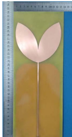
Figure 4. Manufactured bio-inspired antenna.
