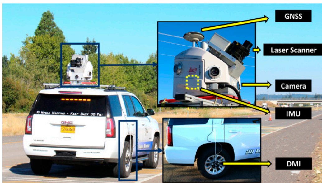
Figure 2. An example of an MLS system (owned by the Oregon DOT) and its components (Leica Pegasus:Two).
