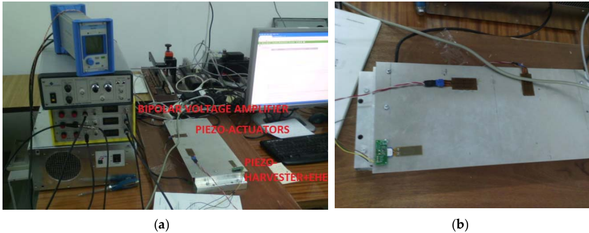
Figure 9. (a) The laboratory stand, (b) the smart plate with piezo-elements (actuators QP10N and harvester V21BL) located on its top surface.
