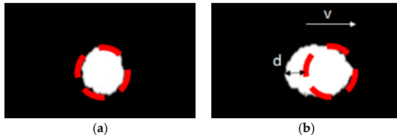
Figure 2. Shape distortion due to motion blur: (a) stopping object; (b) moving object.
