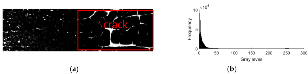
Figure 7. (a) Droplets image of 1.5 \times 10^{-2} cm ink; (b) its grayscale pixel distribution curve.
