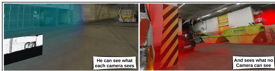
Figure 1. Screenshots from within our application showing that the user gets the supernatural ability to see what each camera can see ( left ), and regions that cannot be seen by the camera system ( right ), both as a colored volume. Using this information the user can change the positions of the cameras by dragging them and see the effect immediately. These capabilities allow users to design camera networks effectively.
