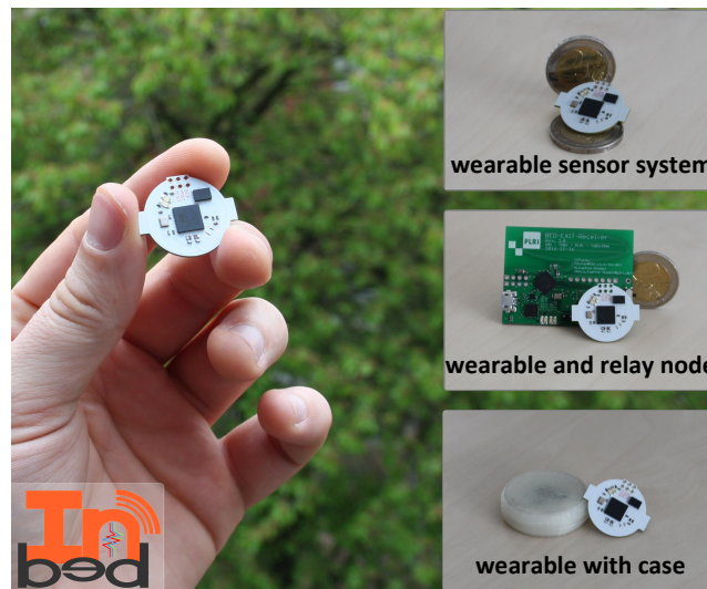
Figure 7. Current INBED wearable board with case and relay node.
