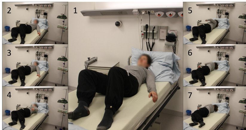
Figure 11. Procedure of a general restless phase, represented by lateral changes of position due to rotations of the test subject with equipped INBED wearable.
