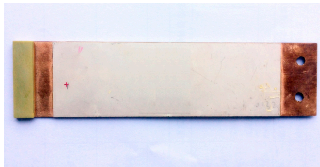
Figure 5. The manufactured cantilever beam.
