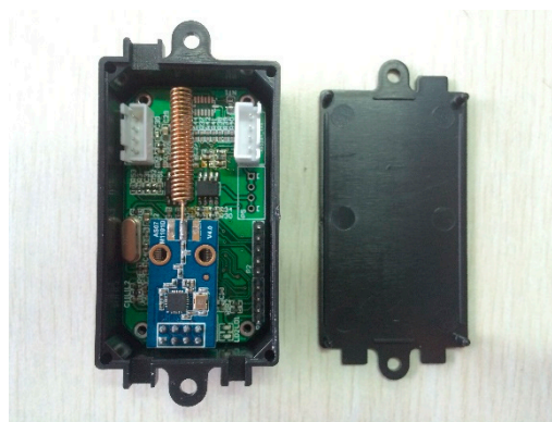
Figure 2. The packaged wireless acceleration sensor.
