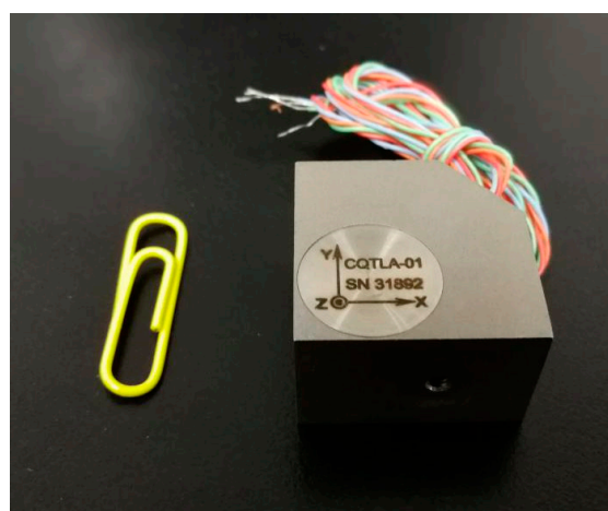
Figure 1. The three-component piezoelectric sensor.
