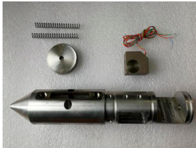
Figure 5. Internal structure diagram of the semi-automatic coupling geophone.
