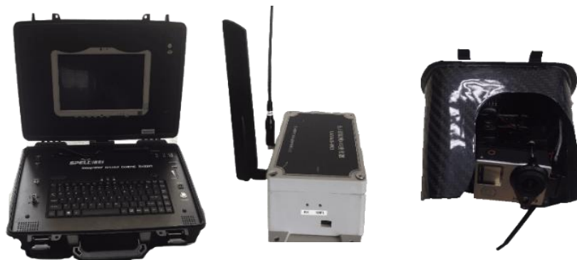
Figure 1. The ground control system, onboard Automatic Identification System (AIS) transceiver and imagery device.
