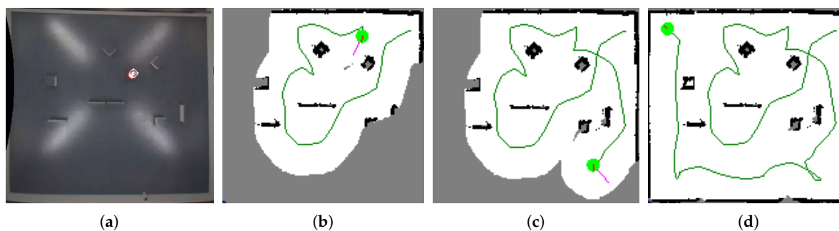
Figure 11. Experiment with a real robot in the SyRoTek system. (a) the robot during an experiment; (b,c) phases of the exploration process; (d) the final map and the performed path.
