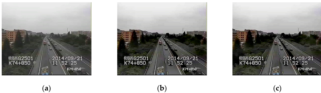
Figure 9. Results of haze removal with and without calibration camera: (a) original image; (b) initial transmission value for calibration camera is 0.596; (c) initial transmission value for image itself is 0.578.
