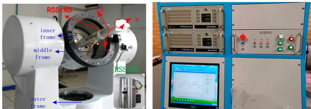
**Figure 10.** Rotating strapdown inertial navigation system (RSSINS) installation on tri-axial rotation table and a console.
