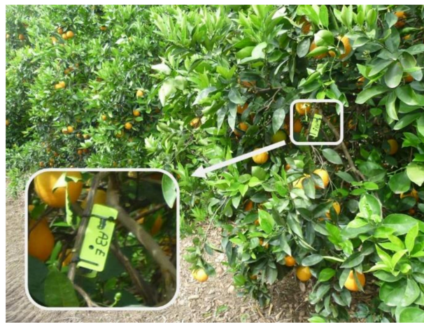
Figure 4. Location of the acceleration sensor on a fruit-bearing branch on the outermost part of the canopy.
