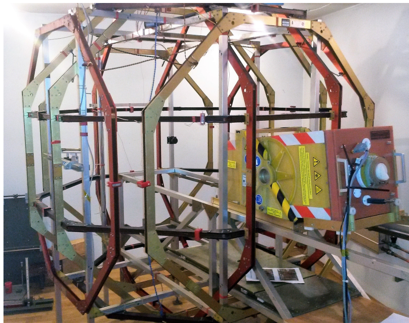
Figure 1. Braunbek coil system of the Magnetsrode calibration facility. The sensor under test is placed inside the yellow measurement box, which is then pushed into the middle of the coil system and set upright for the measurement.
