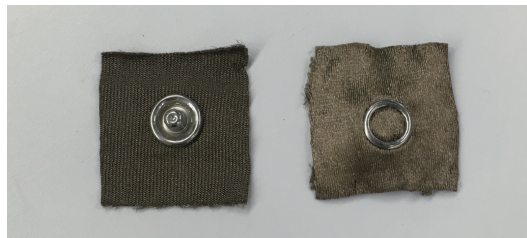
Figure 4. Conductive fabric electrodes where electrode surface contacts skin ( right ) and electrode surface contacts socks ( left ). Electric signals are measured through snaps located at center of electrodes.
