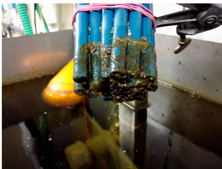
Figure S1. Image of the observed sensor fouling after one week of continuous measurements.
