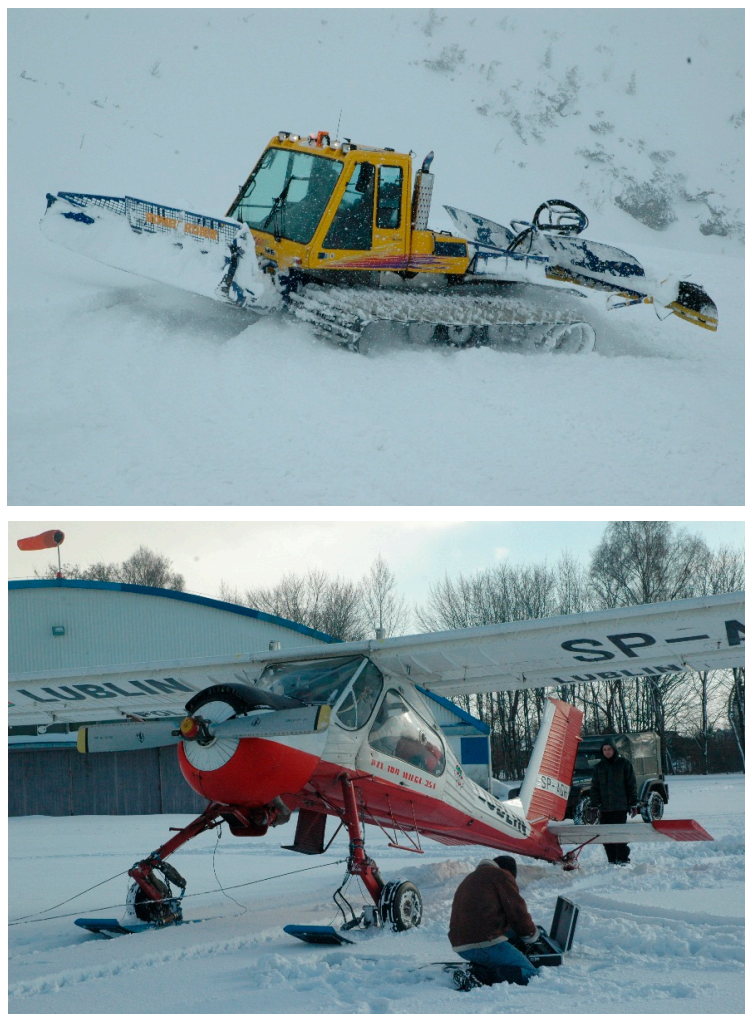
Figure 3. The two machines used in the snow measurements: the Bombardier snow grooming machine (upper photo) and the PZL 104 Wilga 35A airplane (lower photo).
