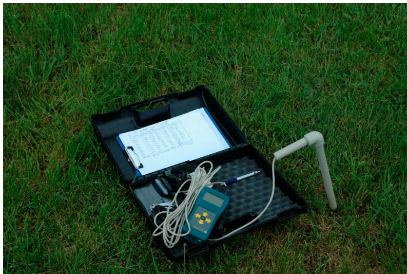
Figure 2. The handheld time-domain reflectometry (TDR) meter used for measurements of soil moisture content of grassy runway.
