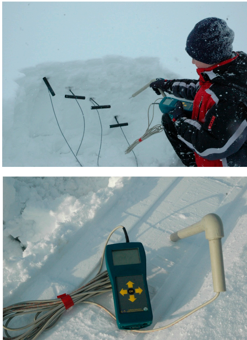
Figure 4. Determining the snow density with the TDR handheld meter: experiment with a grooming machine (upper photo) and with a light airplane (lower photo).
