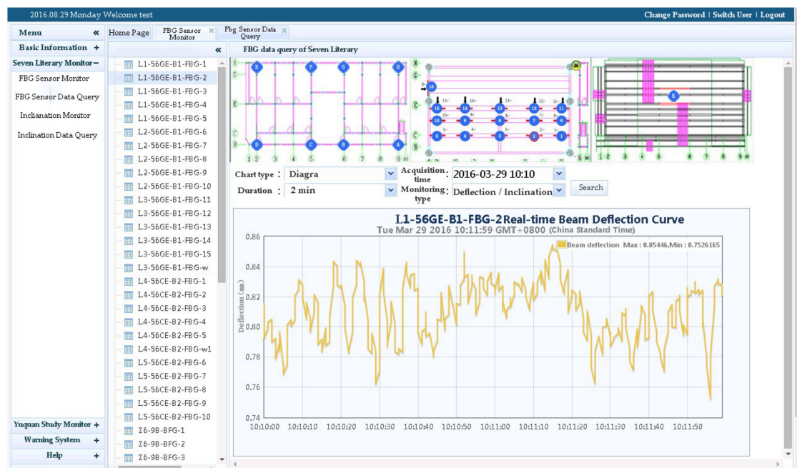
Figure 8. Real-time field monitoring of the ancient buildings via Structural Safety Assessment System server.
