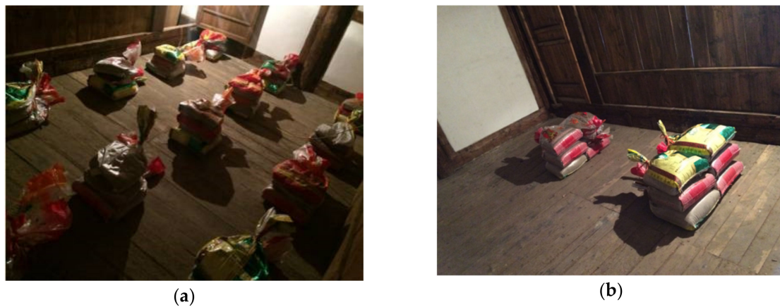
Figure 9. In-situ loading test: (a) Uniform loading; (b) Concentrated loading.
