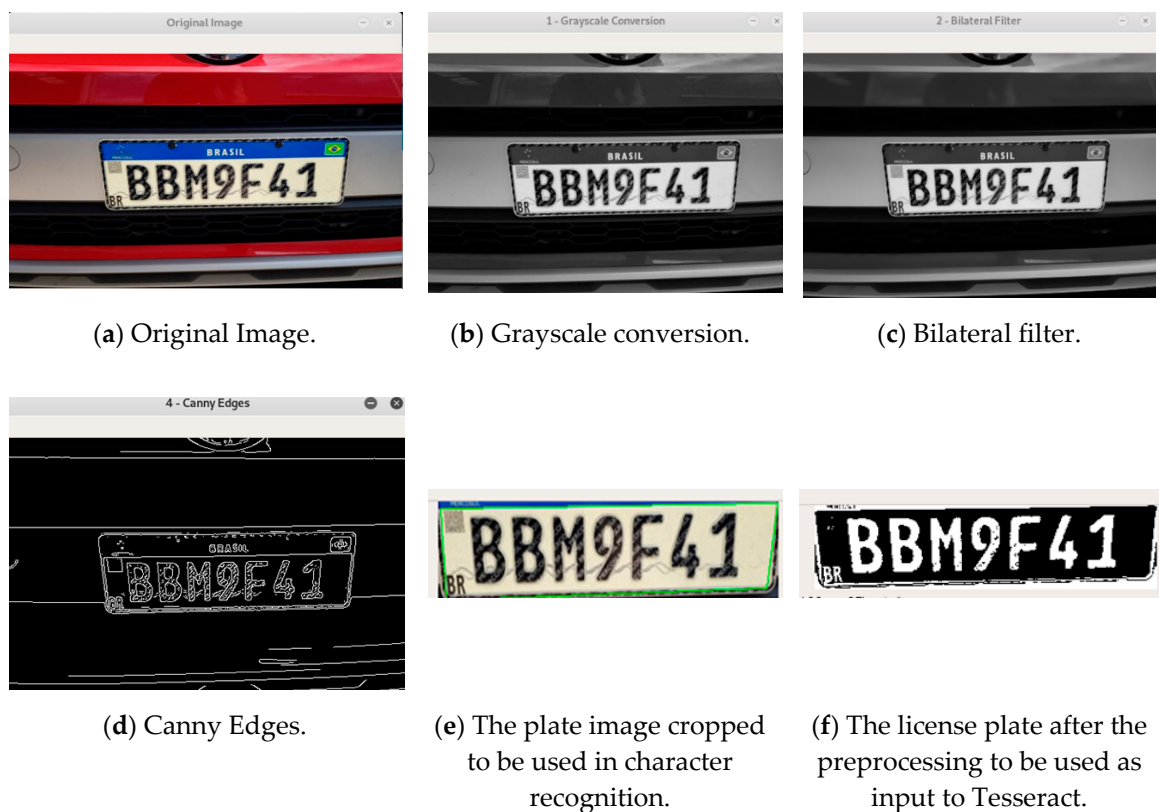
Figure 4. The proposed algorithm applied to the image to detect the characters. (a) Original Image, (b) Grayscale conversion, (c) Bilateral filter applied, (d) Edges detection, (e) The license plate cropped from the main frame, (f) The license plate after the treatment.
