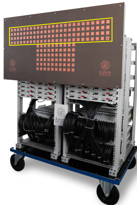
Figure 12. An assembled 100-antenna massive MIMO test bed.
