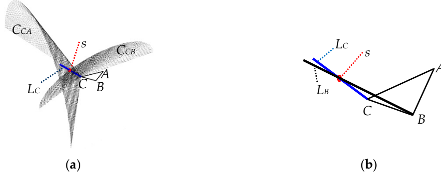
Figure 10. Schematic diagram of 3D-DOA estimation based on the UTA. (a) L_C determined by C_{CA} and C_{CB} . (b) s determined by L_C and L_B .
