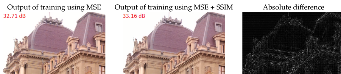
Figure 10. Effects of training with different loss functions ( left : mean squared error (MSE), middle : combination of MSE and structural similarity (SSIM) loss), mostly prominent around object edges ( right ).
