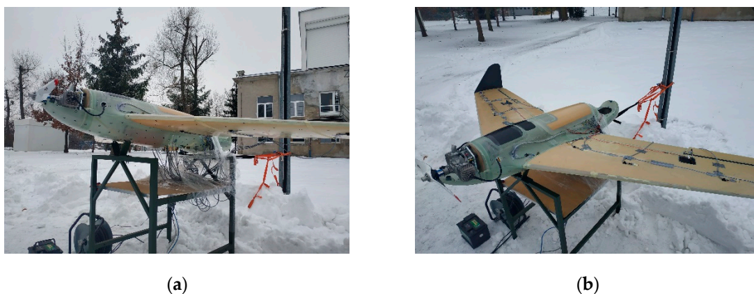
Figure 15. Hornet on the test stand for the engine test (a) bottom view, and (b) top view.
