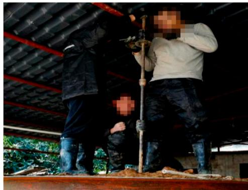
Figure 6. Light dynamic preliminary detector.
