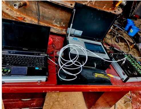
Figure 5. Grouting recorder.
