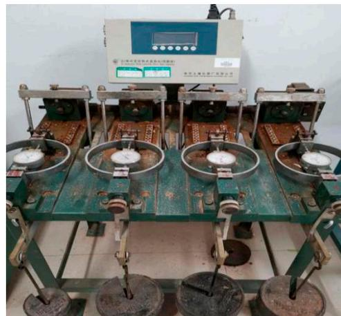
Figure 17. Direct shear test.
