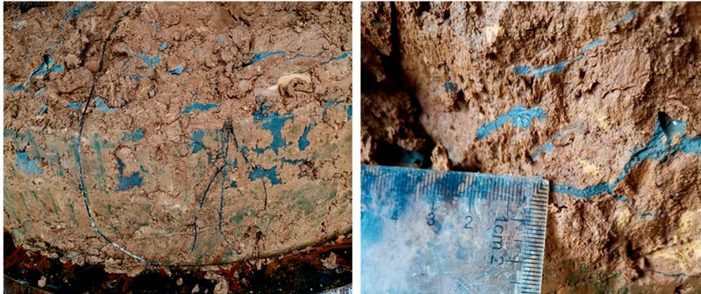
**Figure 12.** Distribution of permeable filling grouting veins.
