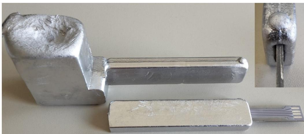
**Figure 4.** The filled cavity without the embedded sensor as well as the embedded sensor separated from the sprue (top right corner) in a detailed view of the protruding substrate.
