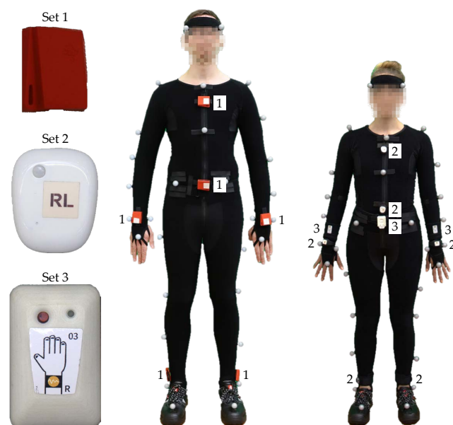
Figure 9. Positions of on-body devices (inertial measurement unit (IMU)) from set 1 (Texas Instruments Incorporated), set 2 (MbientLab), and set 3 (MotionMiners GmbH).
