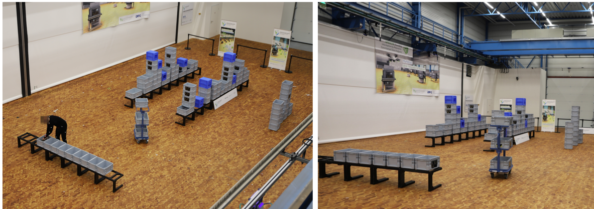
Figure 2. Physical laboratory set-up of logistics Scenario 1—simplified order picking.
