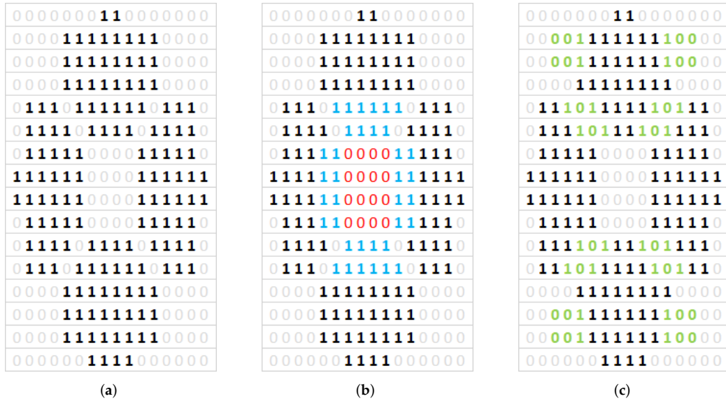
Figure 18. Calculated binary patterns (256 regions) for presented models (Figure 16a) with use of proposed method. (a) generated binary pattern, (b) marked first cascade elements, (c) marked second cascade elements.
