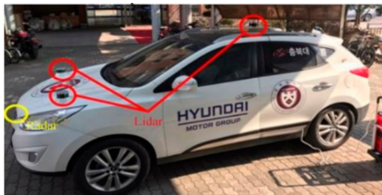
Figure 11. Test vehicle. It was equipped with three lidars and one radar.
