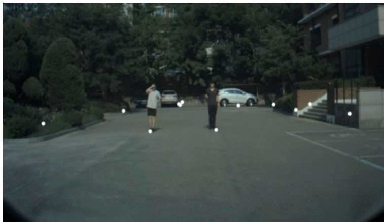
Figure 14. The result of projecting the radar detection result in the image coordinate system.
