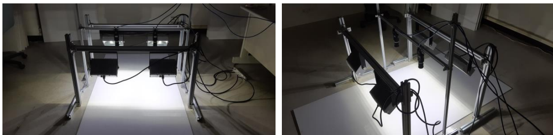
Figure 9. The process of collecting calcium silicate board (CSB) defect samples using the high-speed image capture platform.
