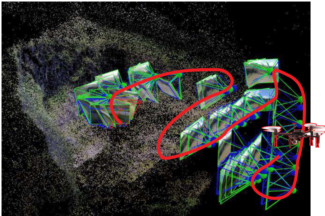
Figure 4. Positions of the cameras during the inspection and the UAV trajectory.
