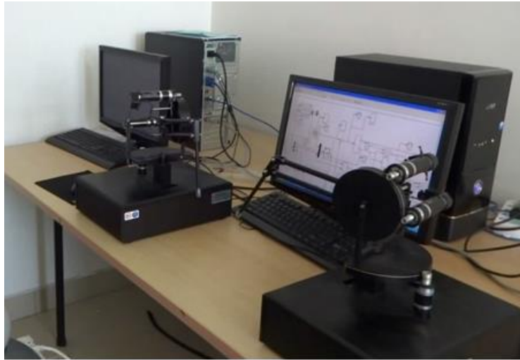
Figure 9. The nonlinear bilateral teleoperation experiment platform.
