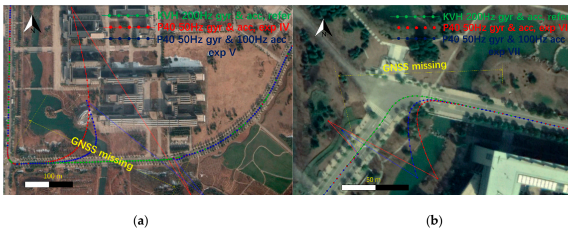
Figure 8. The trajectory of experiments IV to VII projected in Google Earth. The green reference trajectory is from the estimation of GNSS/KVH by the NovAtel IE software, under the GNSS open-sky conditions; the red trajectory is from the estimation of GNSS/IMU-P40 with the 50 Hz gyros and accelerometers by the conventional 15-state Kalman filter, under the GNSS-denied environment; the blue trajectory is from the estimation of GNSS/IMU-P40 with the 50 Hz gyros and 100 Hz accelerometer by our modified Kalman filter, under the GNSS-denied environment. (a) The 50 s GNSS observables missing in straight line; (b) the 30 s GNSS observables missing in turn trajectory line.
