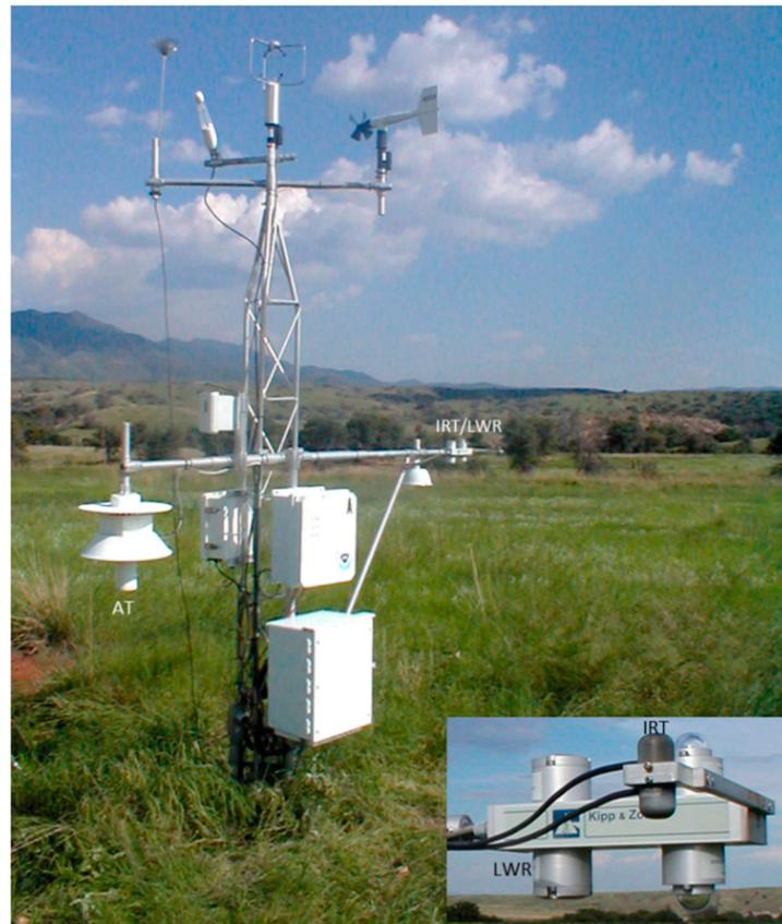
**Figure 1.** Picture of the Surface Energy Budget Network (SEBN) site located in Audubon, AZ. The insert shows Apogee IRTS-P (IRT) and Kipp and Zonen (CNR1-CG3) (LWR) sensors.
