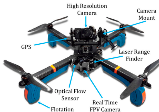
Figure 1. Proposed hardware configuration of bridge inspection UAS.
