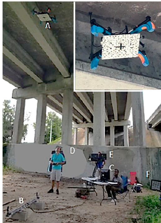
Figure 10. Experimental setup under the US 441 bridge, Alachua, FL. The photograph shows the drone (A), DIC stereo cameras mounted on a beam (B), computer for DIC image acquisition (C), pilot (D), ground station (E), and DIC calibration grid (F).
