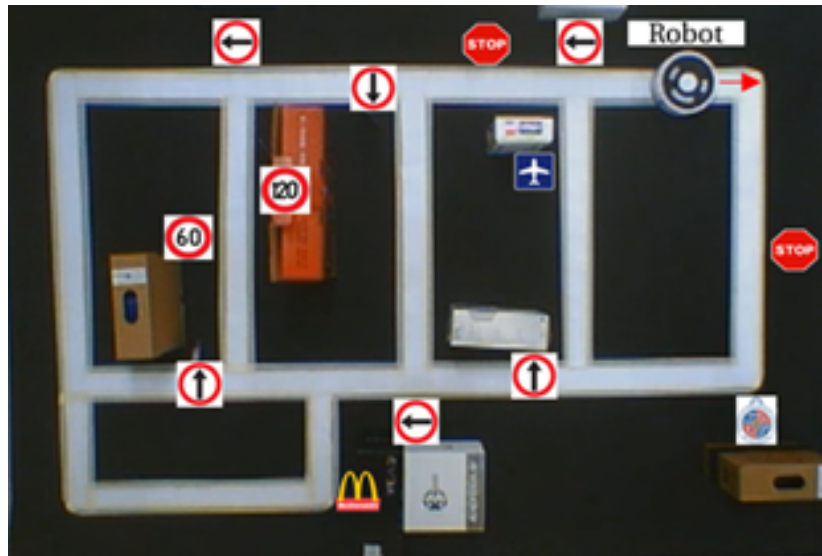
Figure 14. Experimental detection of traffic signals in a real environment.
