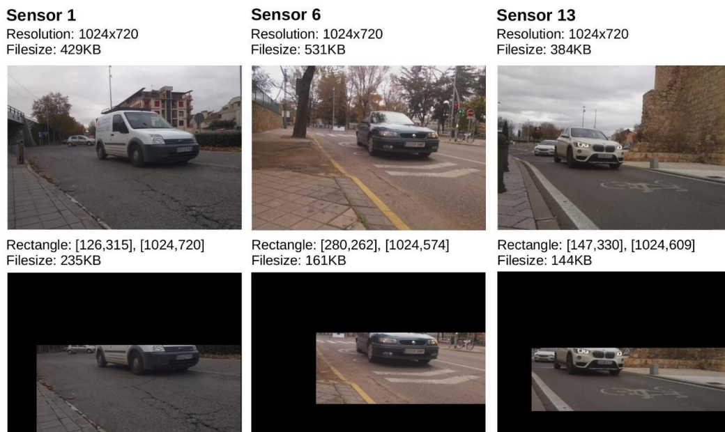
Figure 5. Example of definition of clipping parameters in capture sub-regions in three sensors of the deployed system, with comparative analysis of storage size for each frame. (To protect personal data, the first three digits of the license plate have been blurred).
