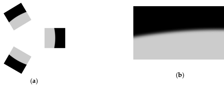
Figure 3. (a) Cluster of three simulated limb images and (b) detail of the edge region highlighting the blur induced by the atmosphere model [9].
