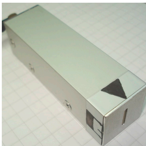
Figure 15. Air-coupled transducer for non-contact reception of evanescent waves.
