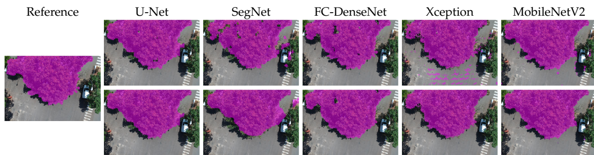
Figure 11. Sample Segmentation 2 prior (first row) and after CRF post-processing (second row).
