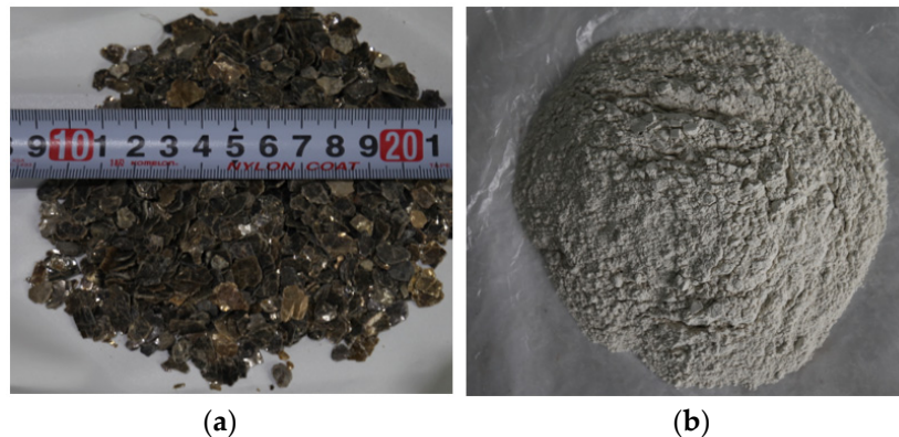
Figure 1. Photos of the expansion-induced materials: (a) vermiculite flake; (b) MgO powder.
