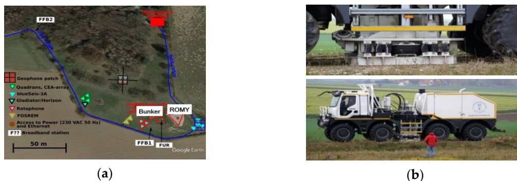
Figure 4. The second part of the Fürstenfeldbruck experiment: (a) scheme of sensors localization during the field test (see chart legend for the FOSREM localization), (b) a view of the VibroSeis truck applied during the experiment.
